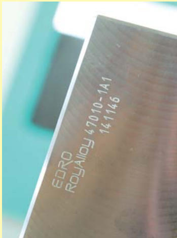
Etching EDRO RoyAlloy™ Heat-number and Customer part number for complete traceability
