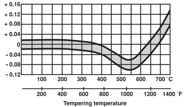
**Note: Dimensional changes during hardening and tempering should be added together.**
