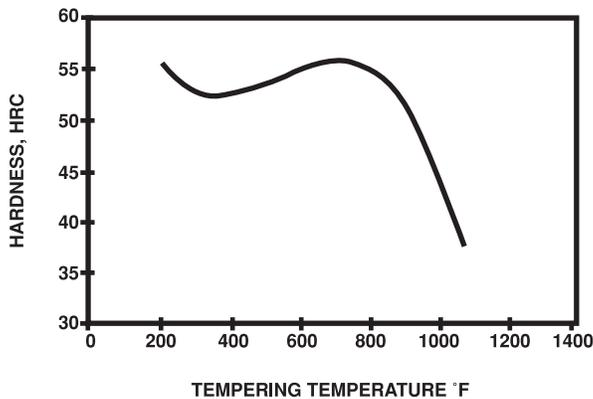
Samples were tempered twice and held at the tempering temperature a minimum of 2 hours. All samples were tested at room temperature.
