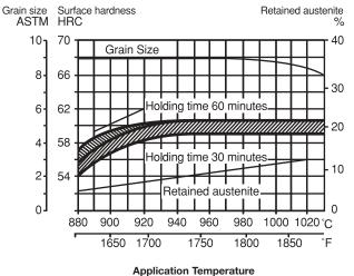
Temperature Soaking\* Hardness before  $\mathsf{F}^\circ$ C° time minutes tempering (HRC) 980 1800 40 52 <u>+</u> 2 390 200 2 56 <u>+</u> 2 570 300 2 57 <u>+</u> 2
