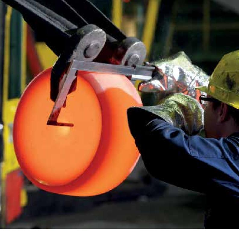
FORGING IS THE NON-CUTTING SHAPING OF METALS
